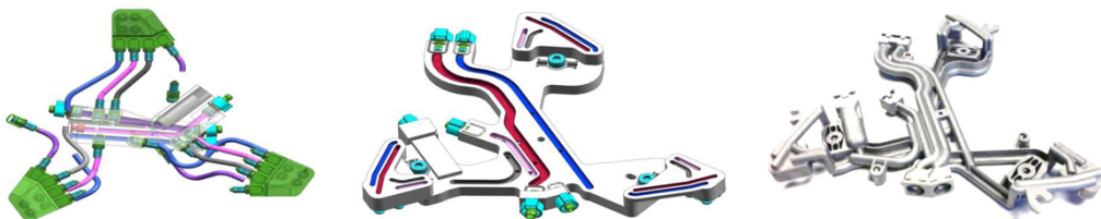
Fig. 55. Three designs of a manifold from the semiconductor industry: conventional design made of PEEK with hoses (110g) (left), monolithic design milled in TiGr5 (200g) (center), and optimized design printed in TiGr5 using SLM (100g) (right). Courtesy of ASML.
