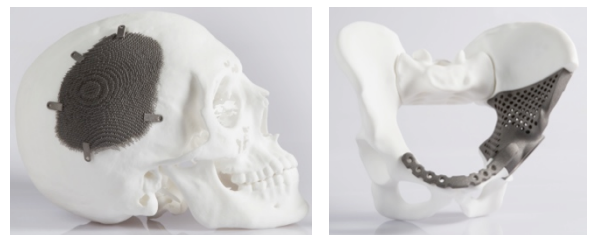
Fig. 18. Titanium implants for the skull (left, [103]) and pelvis (right, [107]) produced using EOSINT M 280.
