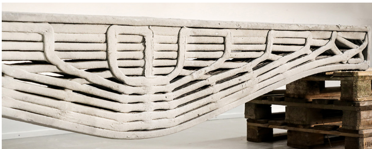
Figure 13 3DLightBeam+ robotic 3D Concrete Printing - Stress-based design for 3D concrete printed horizontal structures, Luca Breseghello, CREATE SDU - Annex A, Case study 011
