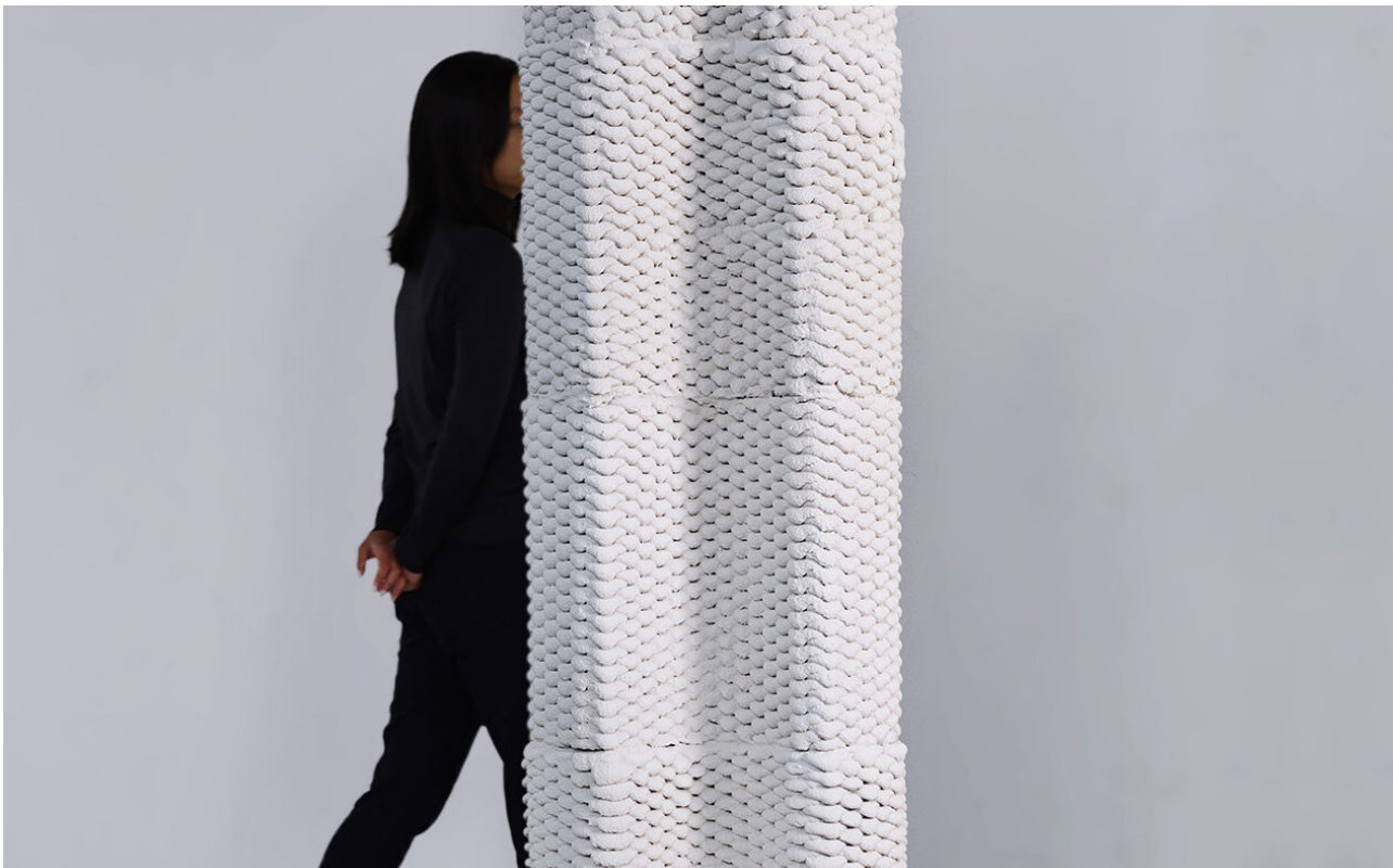
Figure 22 Airlements, Insulated Walls with Sustainable Mineral Foam, FenX, ETH Zürich – Annex A, Case Study 020, Image: Patrick Bedarf, Digital Building Technologies, ETH Zurich
