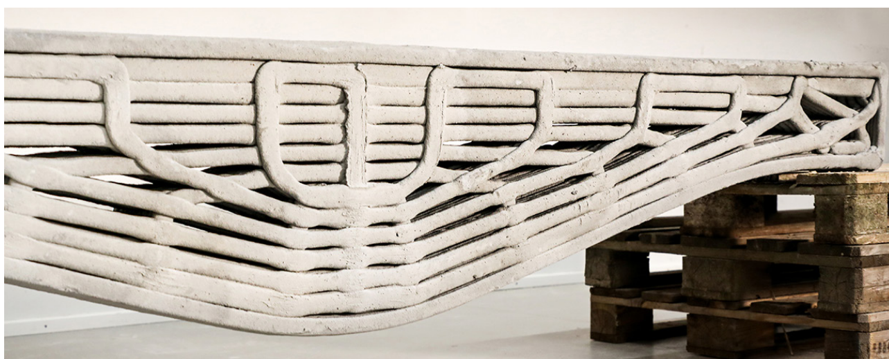
Figure 13 3DLightBeam+ robotic 3D Concrete Printing - Stress-based design for 3D concrete printed horizontal structures, Luca Breseghella, CREATE SDU - Annex A, Case study 011
